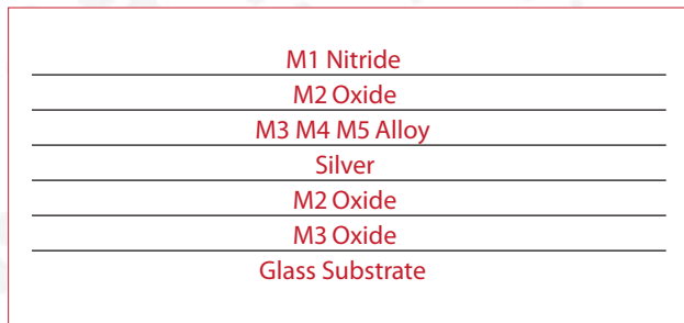
Figure (1) SCHEMATIC STRUCTURE OF A TYPICAL GLASS COATING
